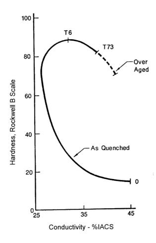
NOTE: Two different hardness conditions can provide the same conductivity reading in %IACS. Use hardness to verify condition.
